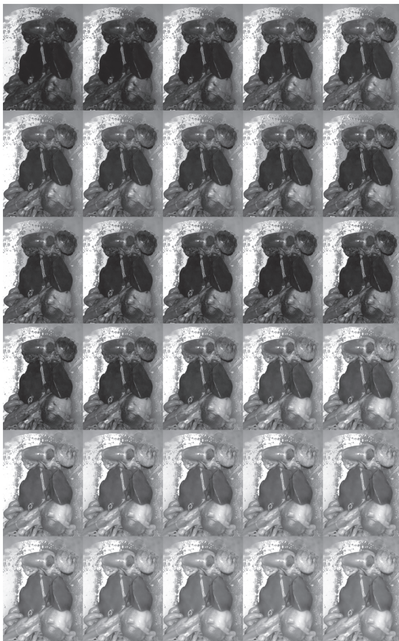
Fig. A.4: Example of an image sweep for a viscera set. Starting at 430nm in the top left corner to 720nm in the bottom right corner.
