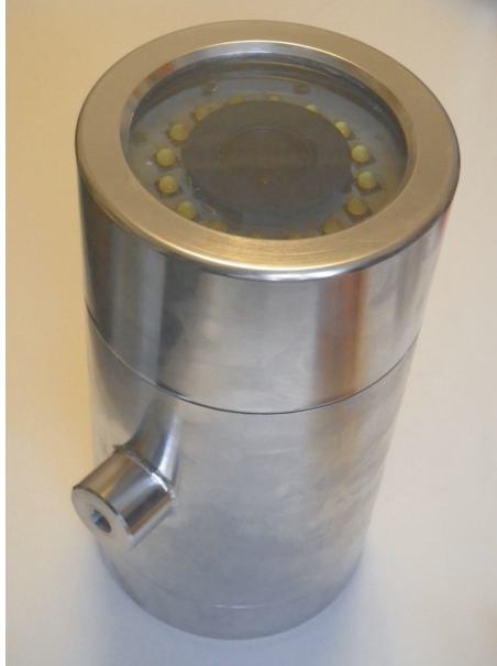
Fig. D.8: The vision tube fitted with camera and LED for another project. The LEDs are fitted on PCB around the lens.
