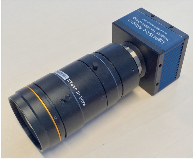
Fig. D.10: ISG camera with Kowa lens mounted.
