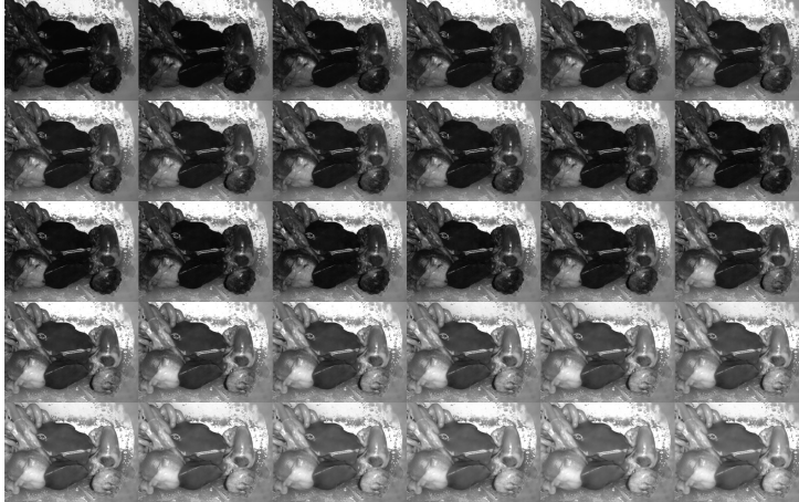
Fig. 3.3: 30 images of a viscera set captured at wavelengths between 430 nm and 720 nm.
