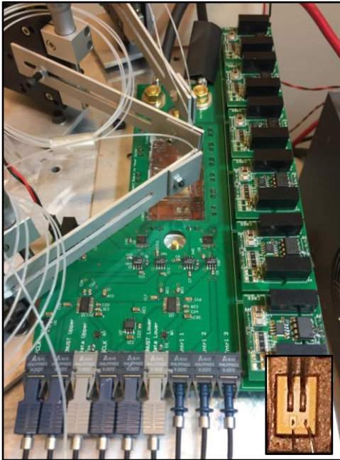
Figure 4. Photo of Measurement Board for SiC MOSFET Power Cycler, including image of MOSFET die from the module.
