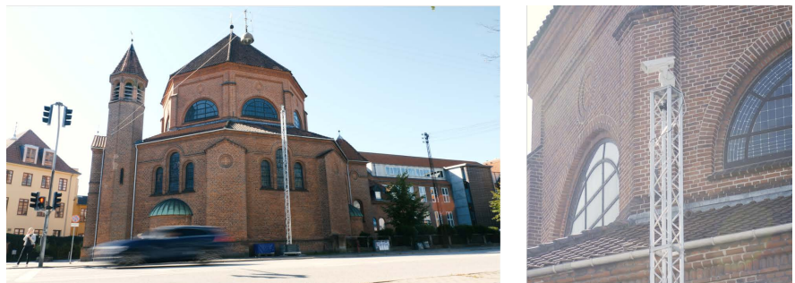
Figure 15. The portable pole deployed at traffic intersection. The pan-tilt motor with one RGB camera is installed on the top of the pole, which makes the RGB camera adjustable remotely.
