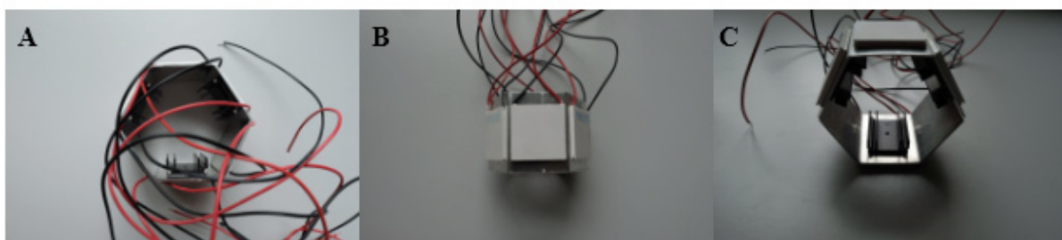
Figure 7: A) Top view of aluminium hexagon tube with the thermoelectric elements attached on the outside, B) Side view, C) Inside view, note the three heat sink radiators.
