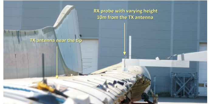
Fig. 17. Setup for experiment 2: 37.3m long blade with downwind side facing up. The TX antenna (OnGround type) is in the front, while the measurement arm with the RX probe is 10 m away.
