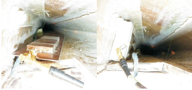
Fig. 18. Three arrangements of the TX antenna: OnGround antenna outside (top), OnGround antenna inside (bottom left) and Vivaldi antenna inside (bottom right).
