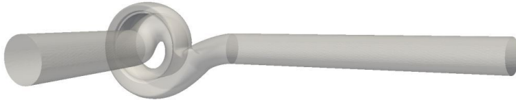
Fig. 5.7: The pump geometry used for the simulation of a rag as it moves through a pump. The pump has a single channel impeller the length of the inlet pipe is three times the inlet diameter and the length of the outlet pipe is eight times the outlet diameter.
