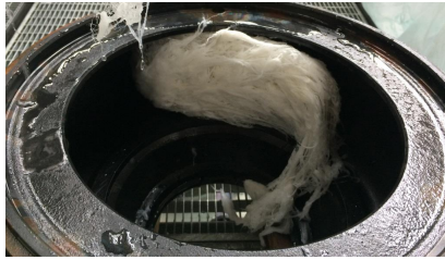
Fig. C.4: Clogging in the cavity after operating the pump at a part load of 60% of the BEP.
