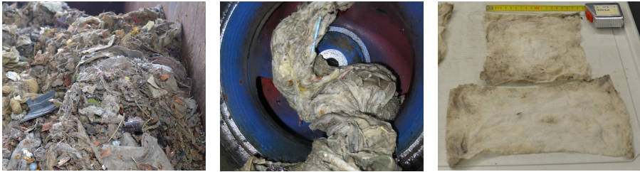
Fig. 1.1: From left to right: Materials from wastewater obtained from the mechanical cleaning stage in wastewater treatment plants, clogged impeller, and example of wet wipes found in wastewater samples (TU Berlin, Chair of Fluid System Dynamics).
