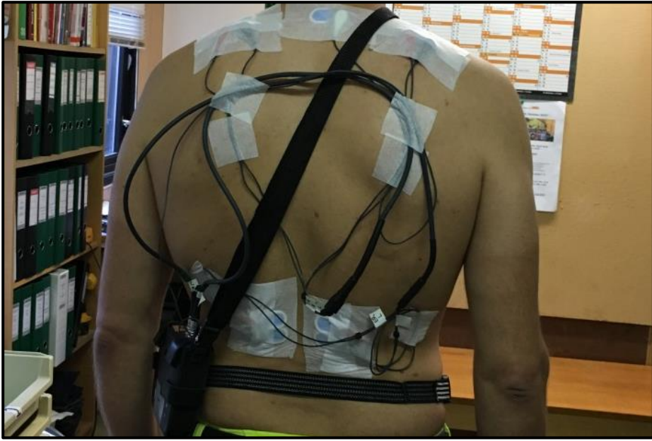
Figure 6: Illustration of the placement of sEMG electrodes.
