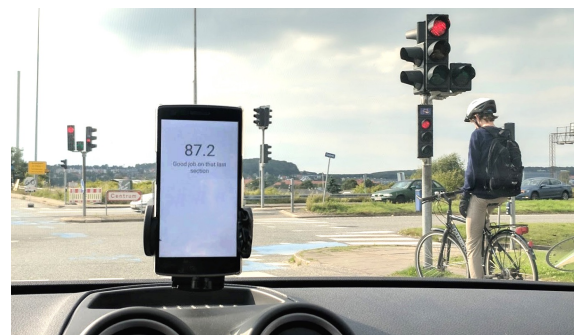
Figure 4. DARA's during-drive feedback presented to the drivers every time the car is stopped, after driving at least 600 meters.
