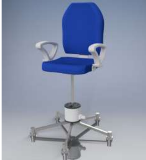
Fig. 1. Illustration of the designed instrumented office chair enabling the recording of sitting postural control characteristics.
