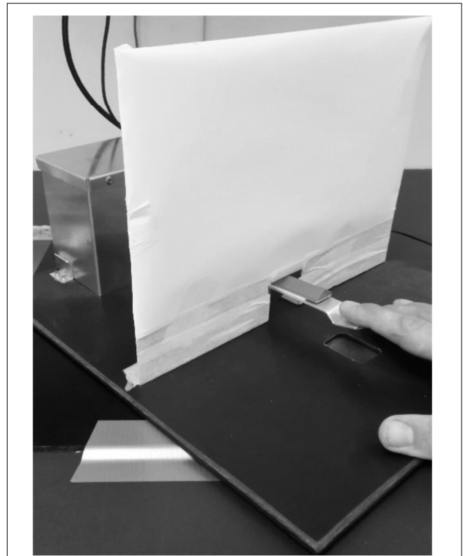
FIGURE 2 | Illustration of the custom-built passive tapping machine.
