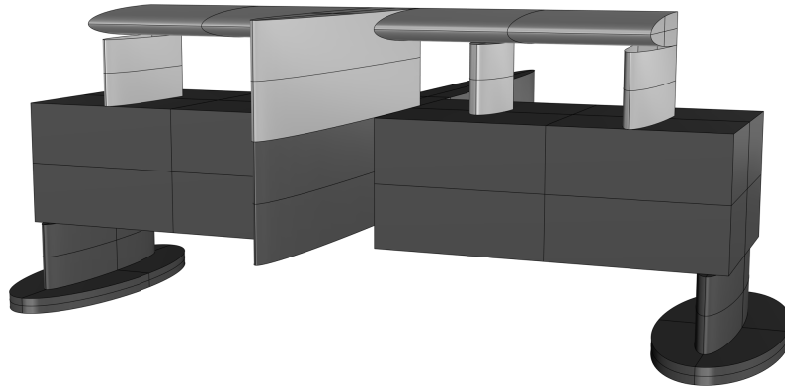
Fig. 2.8. Illustration of the simplified geometry used for calculation of drag coefficients. The dark color resembles the geometry below the SWL, while the light grey color resembles geometry above.
