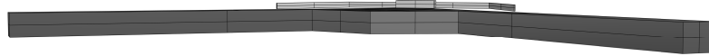
Fig. 5.8. Illustration of the simplified geometry used for calculation of drag coefficients. The dark color resembles the geometry below the SWL, while the light grey color resembles geometry above.
