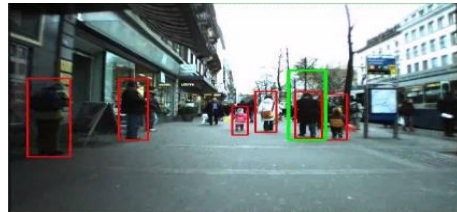
Figure 1. An example detector failure for the pedestrian of interest. Green box denotes detector result where red box denotes ground truth.
