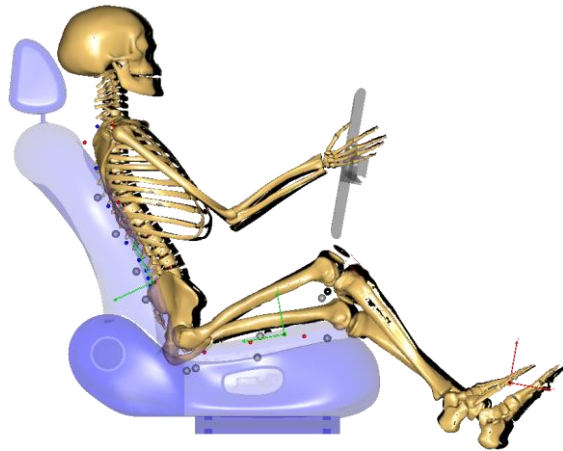
Figure 4. Overlaid image of initial (pedal force = 0 N, color black) and final (pedal force = 200 N, color yellow) postures. The muscles have been graphically removed from the figure in the interest of legibility.
