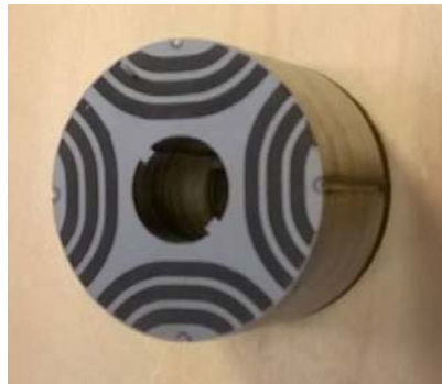
Fig.3.2_3 Rotor prototype manufactured with moulding technology [8].
