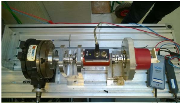
Fig.3.6.2_2 Experimental setup for torque performance measurement [8].
