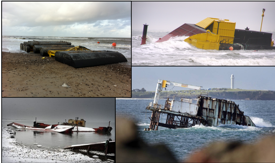
Fig. 1.11: Examples of strandings of WECs due to mooring failures. Pictures adapted from Nordyske (2011); Illawarra Mercury (2015)
