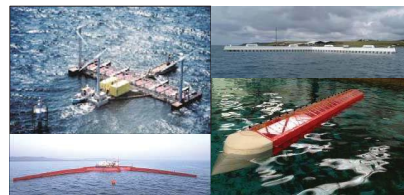
Figure 1: Large floating WECs with passive mooring systems. Top left is Floating Power Plant (2015), top right is LEANCON Wave Energy (2015), bottom left is Wave Dragon (2015) and bottom right is KNSwing .
