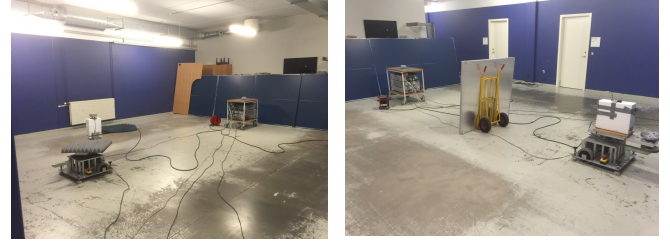
Figure 4. A photo of the LOS scenario (Biconical antenna as the Rx antenna) and the obstructed LOS scenario (Horn antenna as the Rx antenna).
