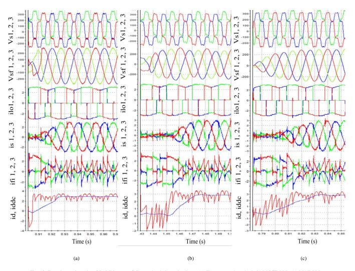
Fig. 12. Experimental results of SAPF in case of distorted unbalanced voltage. (a) The proposed method. (b) MCCF-PLL. (c) MAF-PLL
