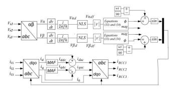
Fig. 7. the proposed methodology of harmonic control method.
