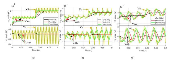
Fig. 3. Performance example of MAF at  $T_w = 0.02s$ , 0.01 and 0.02/6s. (a) Existence of harmonics of the order  $6h \pm 1$  in the grid voltage. (b) Unbalanced and contaminated grid voltage. (c) Existence of harmonics and dc offset.
