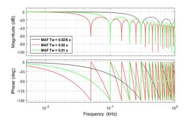
Fig. 2. Bode plot of MAF at  $T_w = 0.02s$ , 0.0s1 and 0.02/6s
