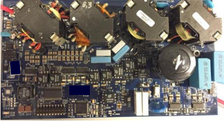
Fig. 2. Photo of the built PV microinverter prototype.
