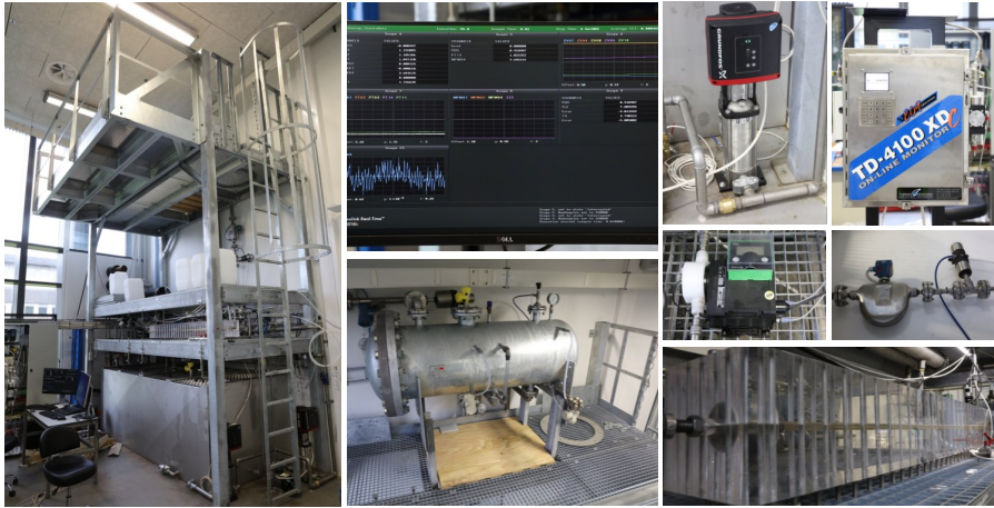
Fig. E1: Photo of the set-up showing from left top: Riser platform, Simulink Real-Time target PC interface, reservoir water pump, TD-4100, three phase Gravity separator, oil pump, Coriolis flow meter connected to a valve, PMMA transparent hydrocyclone.
