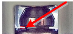
Fig. 15. Gap occurring in the coupling of the servomotor and the valve piston.
