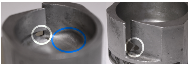
Fig. 2.6: Cavitation on the cylindrical section of the hydrocyclone, marked with white and blue colour, the shown example is from a used Vortoil hydrocyclone, which is the same type as used in the scaled pilot plant described in Appendix part III.
