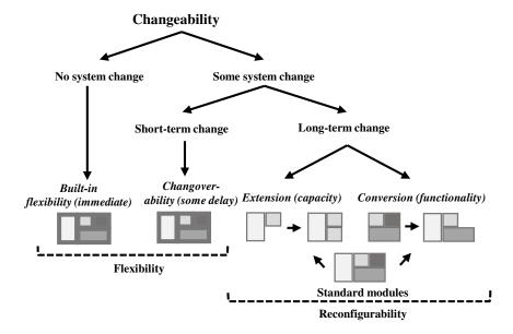
Figure 8. Manufacturing system reuse strategies for different changeability types. Combined from the work of Benkamoun et al. (2015) and Jørgensen (2013).
