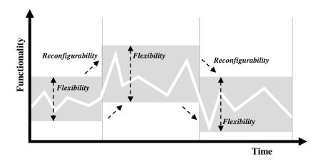
Figure 2. Changeability as a combination of flexibility and reconfigurability.
