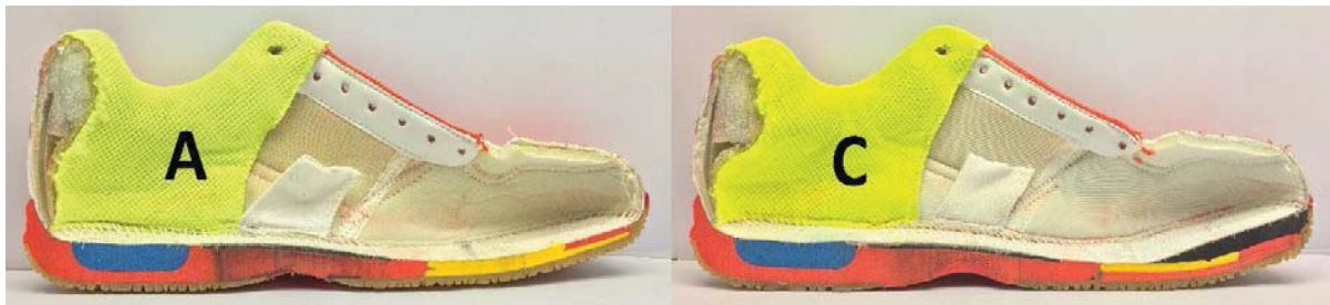
Figure 1. Sagittal cut trough of the 0 (A) and 8 mm (C) shoes. The wedge is observed as the black part on top of the base sole for shoe C; shoe B was similar with a wedge of only half this height.
