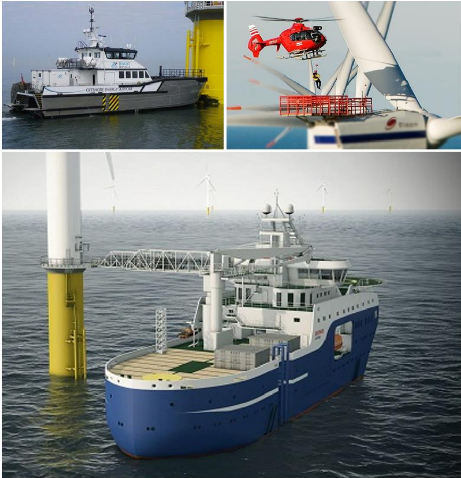
Figure 1-15 Example of access vessels: CTV top left, helicopter top right and SOV in bottom (offshorewind.biz)
