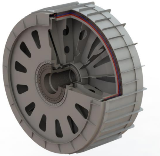
Figure 4-3 – 20MW PDD generator concept model
