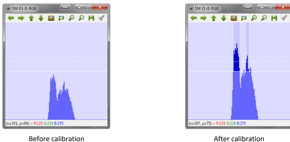
Figure 25 | Histograms are used to adjust the detector. If the amount of activity is sufficiently high, so that the software recognizes it as a road user, the activity is marked with a bright colour (in this case blue). If the parameters of the detector are not adjusted correctly, then the road user will either be missed or only partly detected (left). After the adjustments of the parameters the road user will be clearly detected (right)
