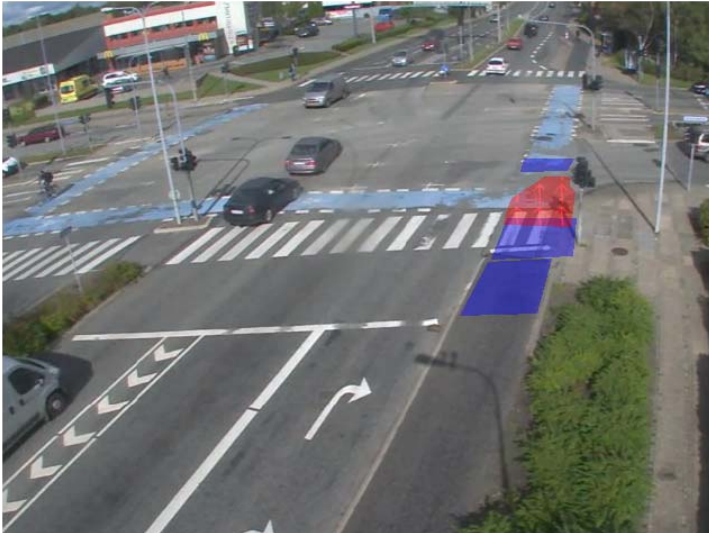
Figure 15 | Example of the design of detectors in the module for straight going cyclists. The module consists of three edge detectors (blue) and one flow detector (red)
