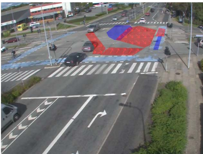
Figure 17 | Example of the design of detectors in the module for left turning vehicles. The module consists of two edge detectors (blue) and four flow detectors (red)
