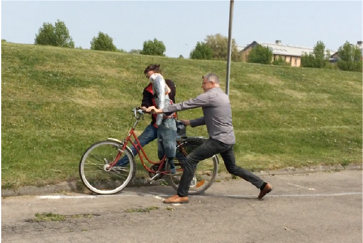
Figure 6: Simulating sideways cycling accident with a crash test dummy.
