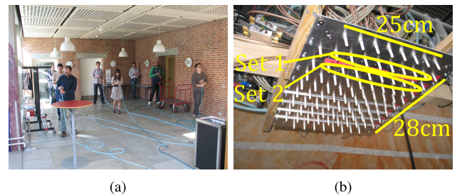
FIGURE 1. Scenario and array shown in the results. (a) Scenario with spread users in NLoS, S-NLoS. (b) Compact 2D array, C2D.
