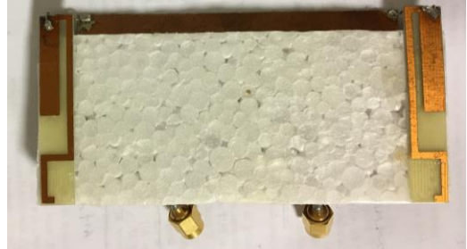
Fig. 3. Photo of the mockup handset antenna.
