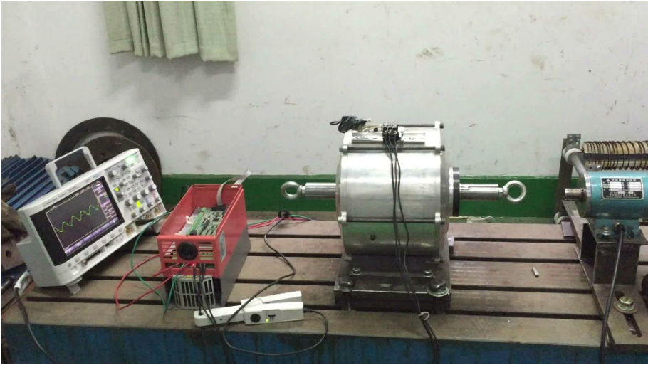
Figure A-19 No-load test
