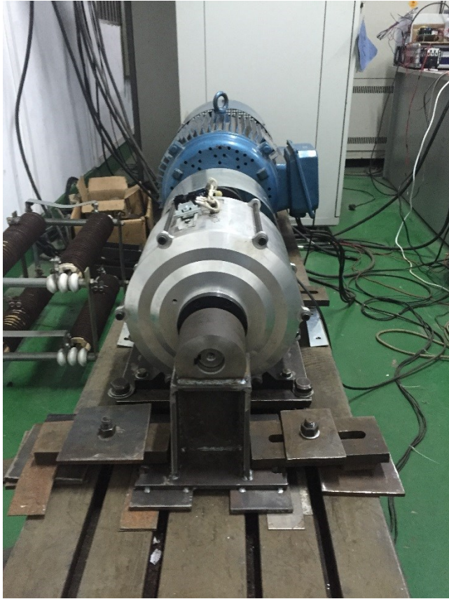
Figure A-21 Stall torque test
