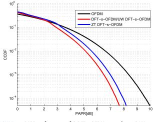
FIGURE 10. PAPR performance of G-DFT-s-OFDM, assuming 16QAM modulation.
