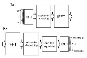
FIGURE 1. Structure of G-DFT-s-OFDM baseband transceiver.
