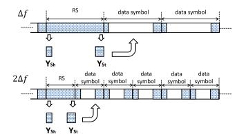
FIGURE 5. Proposed reference sequence mapping for UW DFT-s-OFDM.
