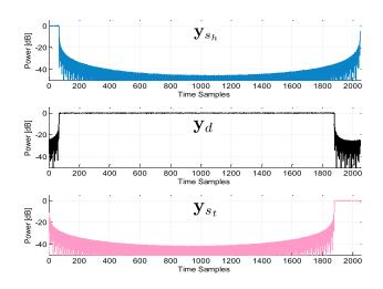
**FIGURE 2.** Components of a G-DFT-s-OFDM signal, assuming N=1200,  $N_{s_t}$ =144,  $N_{s_h}$ =17,  $N_{FFT}$  = 2048. The component  $y_d$  represents a ZT DFT-s-OFDM signal.
