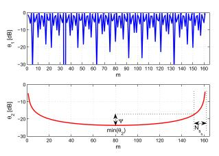
**FIGURE 3.** Oscillating part and envelope of the leakage, assuming N=1200,  $N_{FFT}=2048$ ,  $N_{S_0}=161$ .
