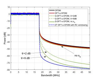
FIGURE 11. Ouf-of-band emissions of G-DFT-s-OFDM.
