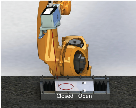
Fig. 1. A KUKA Quantec KR 120 R2500 pro mounted with an Arges remote welding elephant head. On a closed contour processing can start at any point. On an open contour processing can start either in point A or B.
