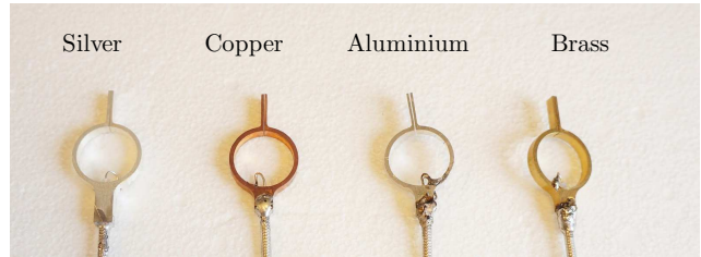
Fig. 10. Loop antenna mock-ups made out of four different materials with embedded air-capacitors.
