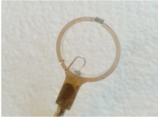
Fig. 7. Detailed picture of the silver antenna showing the structure without using tin to fix the tuning capacitor or the feed.
