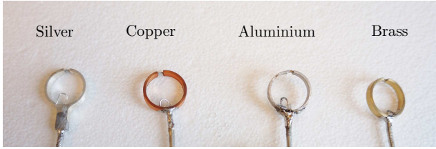
Fig. 6. Loop antennas made out of four different metals tuned with 2.7 pF fixed capacitors.
