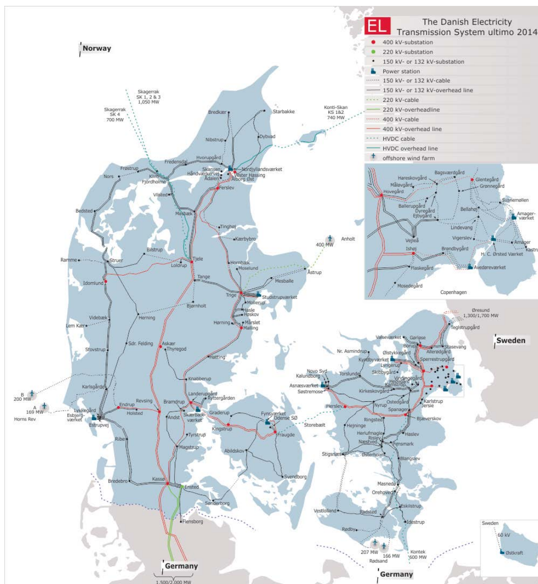
Figure 1: Overview of the Danish Electricity Transmission Network
