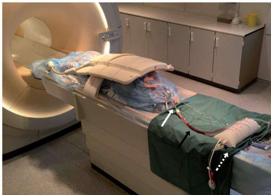
Fig. 3. Experimental set-up. A pig is lying on the flat bed in the MRI scanner. It is wrapped in plastic to avoid risk of contaminating the scanner. On top of the pig is the coil. On the green cloth is the tube with the PE suspended in saline (black arrow). Attached are the cannula with a plastic clamp (white arrow) and the MRI-safe pressure bag (dashed white arrow).
