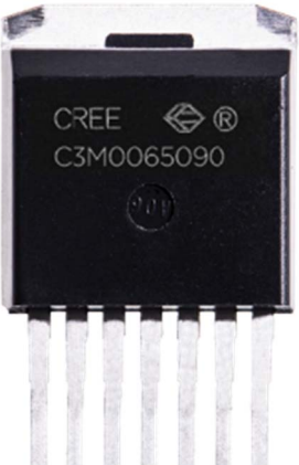
Fig. 7: D2Pak package MOSFET from CREE and the parameters.
