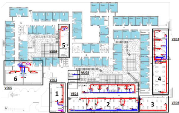
Figure 2 All the offices are naturally ventilated (in light blue), and the rest common rooms are ventilated by six ventilation units (marked in numbers)
