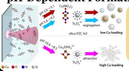
Low and medium solution pH: ablated silica clusters (oxidized silicon atoms upon interaction with water) are protonated, repel nearby Cu2+ ions, resulting in low wt.% loading of Cu, and Cu-core/silica-shell morphology
