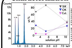
Representative SEM-EDS spectrum of Cu-silica-10.4 sample. Inset shows wt.% Si, O, and Cu quantified in samples fabricated from different pH
