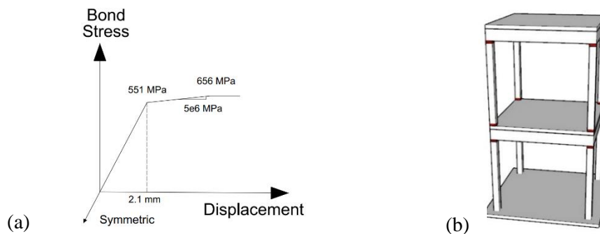
Figure 5. (a) Bond stress versus slip displacement model and (b) locations of zero length section elements.
