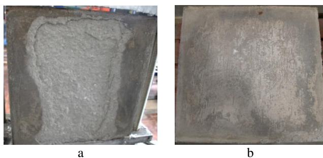
Figure 14. Specimens after the fire-induced spalling tests. a) plain concrete b) RTPF reinforced concrete.
