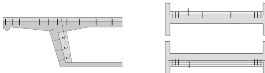
Figure 6. Reinforcement and strengthening of a) concrete bridge b) building slab
