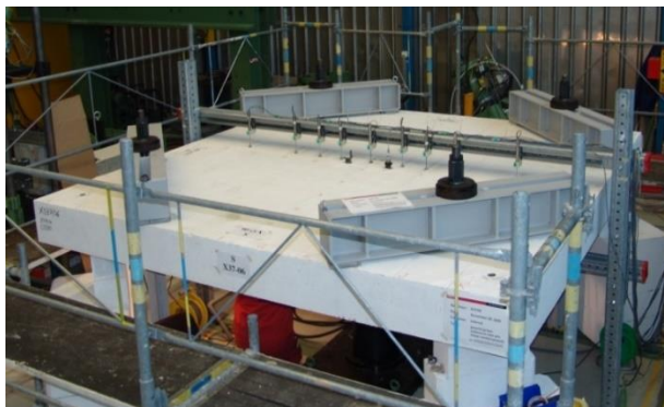
Figure 18. Punching shear test setup
