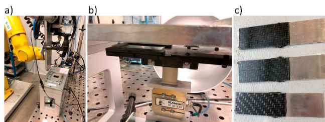
Fig. 4. (a) joining cell; (b) pressure jig detail; (c) samples of Al 7075 – Tepex 102 joints.
