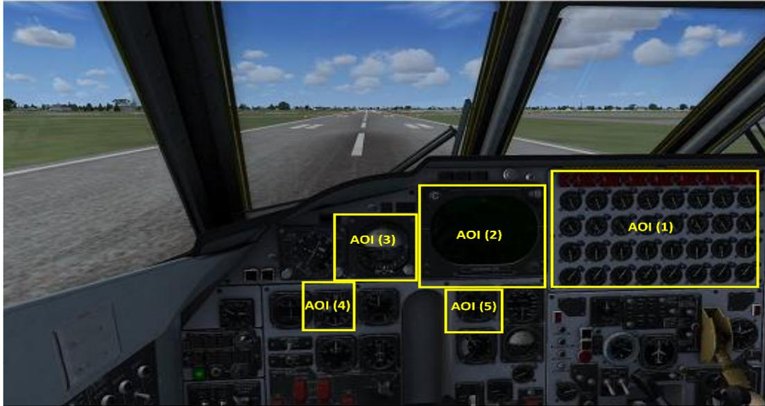
**Figure 4.1. AOI of B-52 Cockpit display: (1) Engines indicators; (2) Enhanced visual screen (3) Attitude indicator; (4) Altimeter; (5) Airspeed indicator.**
