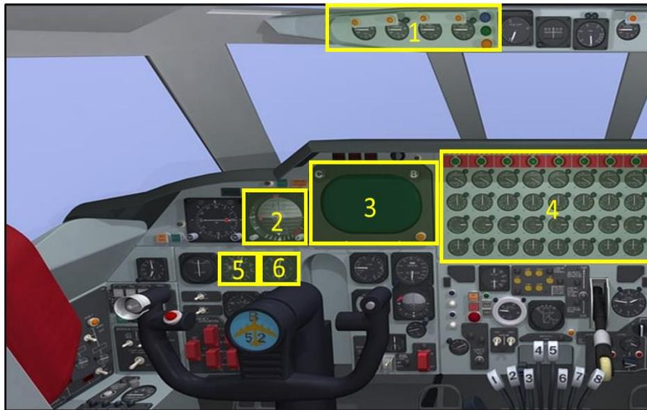
**Figure 3.2. Cockpit display (B-52) with associated important AOIs: (1) engine oil pressure; (2) attitude indicator; (3) enhanced visual screen; (4) engines indicators; (5) altimeter; (6) airspeed indicator.**
