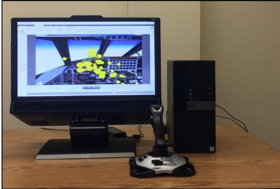
**Figure 3.1. Experimental set up. Windows workstation with a Tobii TX300 eye-tracker in the Microsoft light simulator software (FSX) Human Factor Lab at the University of Oklahoma.**
