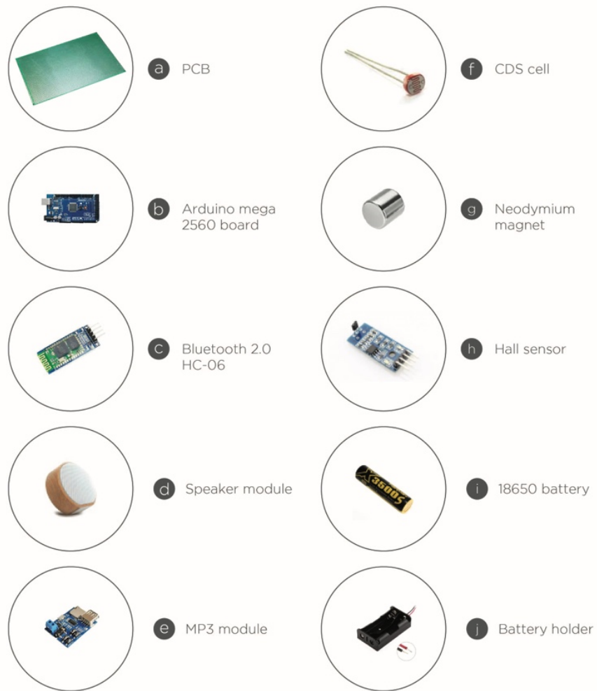
Figure 20. Internal components of prototype
