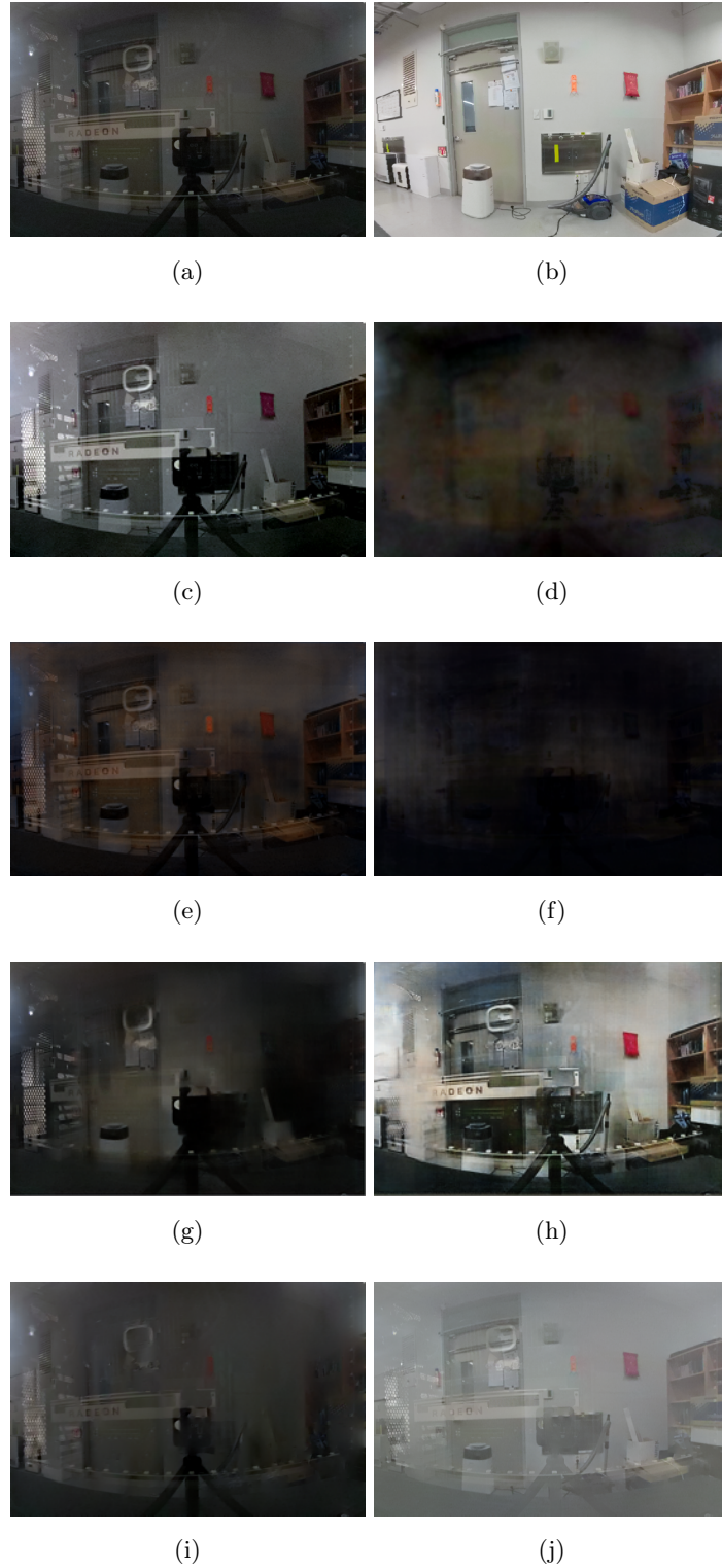
Figure 24: Experiment results of comparison. (a) Glass image, (b) Reference image, (c - d) T and R of [2], (e - f) T and R of [3], (g - h) T and R of [4] and (i - j) T and R of Proposed method.
