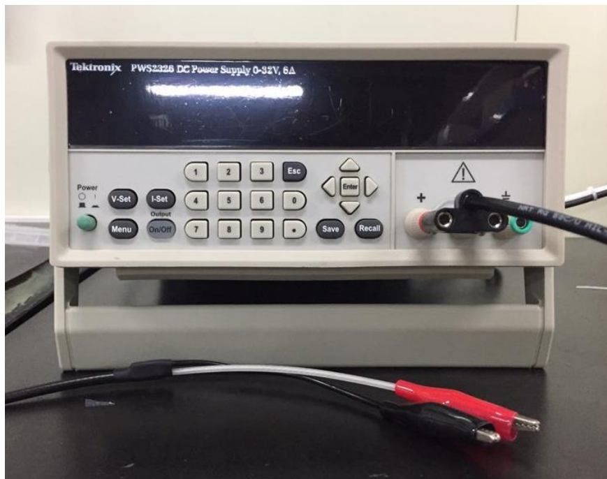
Figure 25 DC power supply was used for applying an electric stimulus to the pixelated mechanical metamaterial.
