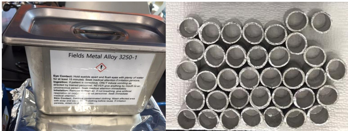
Figure 17 Field's metal was melted on the hot plate with a temperature of 130°C for 30 minutes. Liquid LMPA was then poured into the silicone mold to fabricate the cylindrical LMPA layer.
