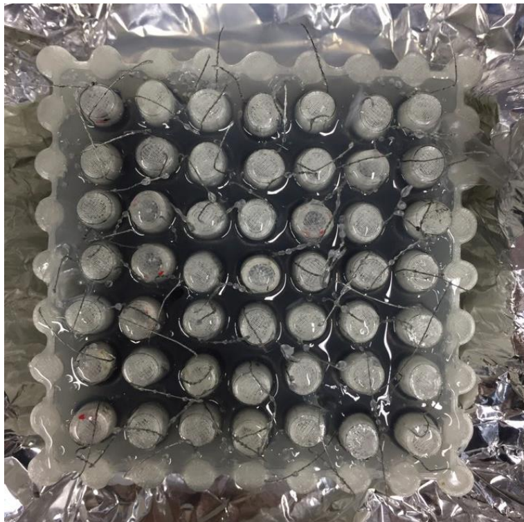
Figure 19 Liquid silicone rubber was poured into the mold after putting all pillars into the cavities in the bottom of the mold. To remove air bubbles, the mold was placed in the vacuum chamber for 25 minutes. After degassing, the mold was placed on the hot plate at 65 °C for one hour to cure the silicone rubber.
