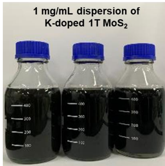
Figure 1.3. Digital image of K doped 1T MoS 2 dispersion in DI water, which indicates that scalable synthesis of K-doped 1T MoS 2 is possible.
