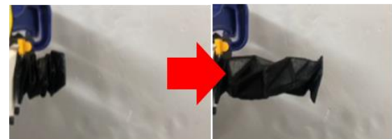
Fig II.2.10 Hybrid actuating modules based on origami structures
