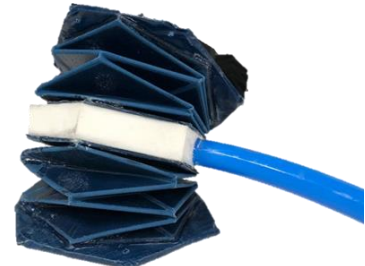
Two modules linked through the hose coupling
