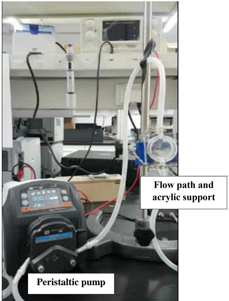
Figure 44 Experimental setting for flow rate determination
