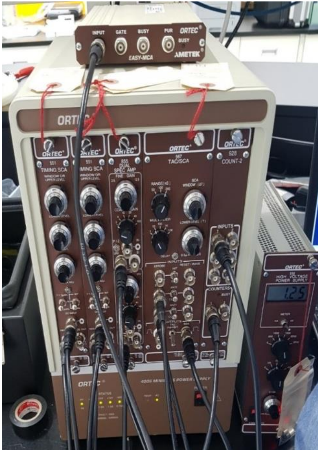
Figure 33 The actual experimental settings of the coincidence circuit based NIM module
