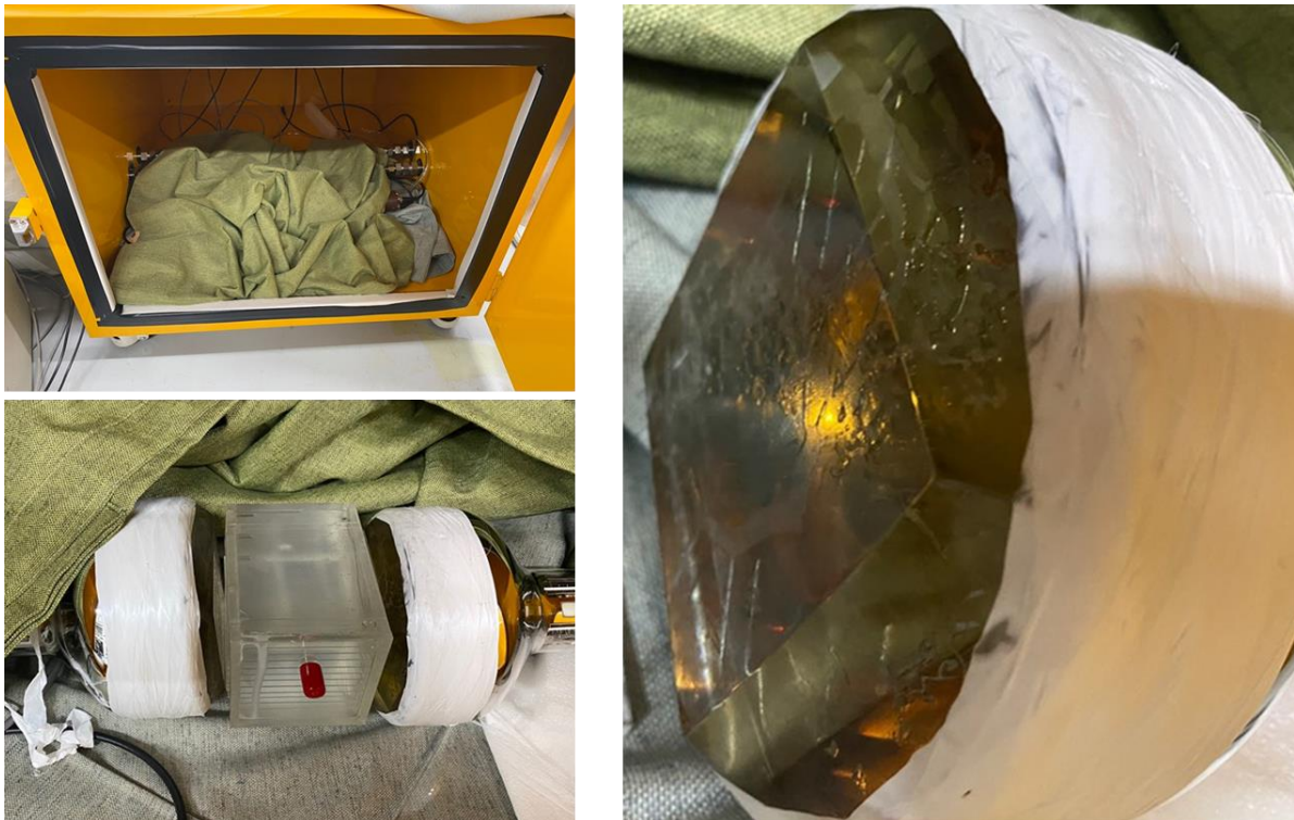
Figure 79 Detection preparation with detection chamber, light guide, and PMT in lead shield
