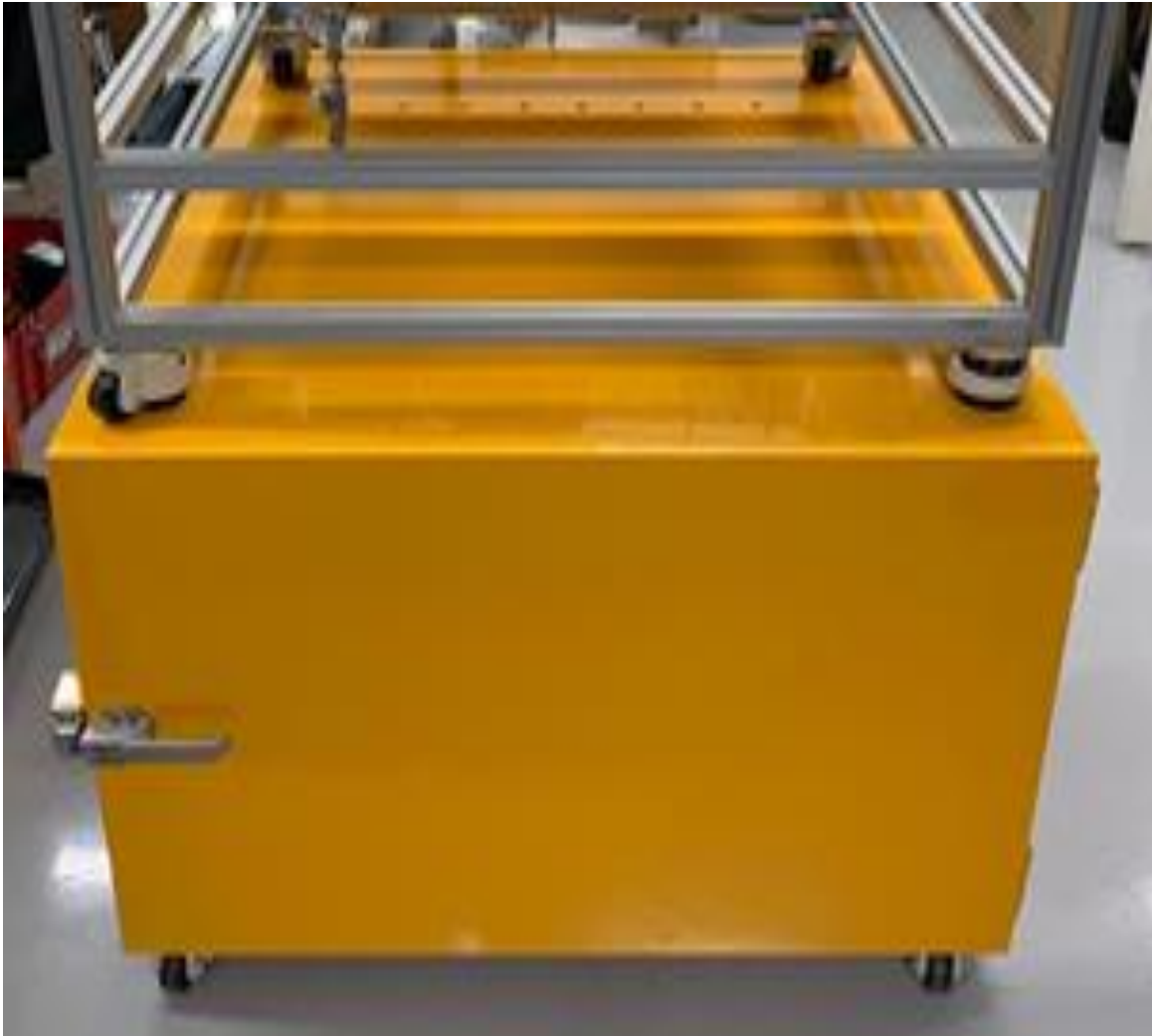
Figure 40 External view of lead box for shielding background radiation
