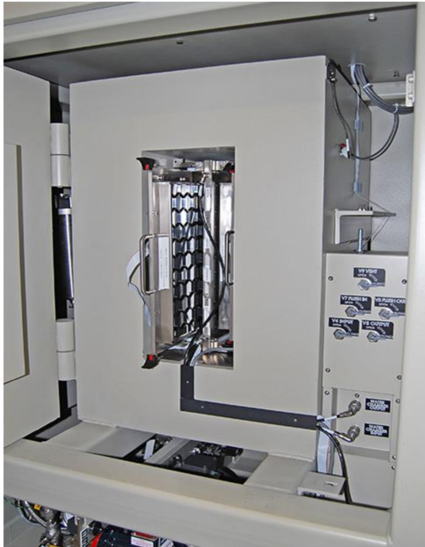
Figure 11 Entire system for performance of a low activity beta-sensitive ^{90}\text{Sr} water monitor
