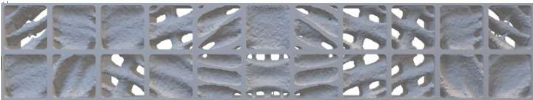
Figure 2.5 Lattice structure of simply supported beam example
