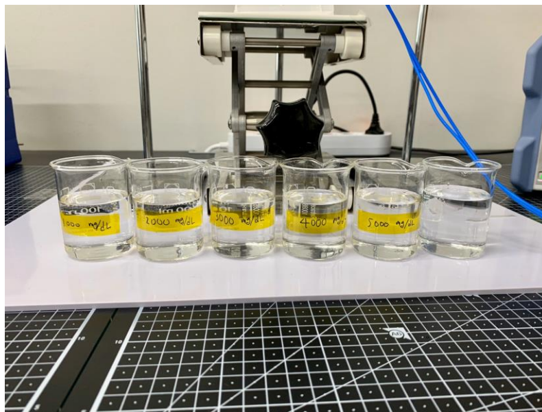
Fig. 2-10. Glucose, DI water solution from 50 to 300 mg/dl concentration
