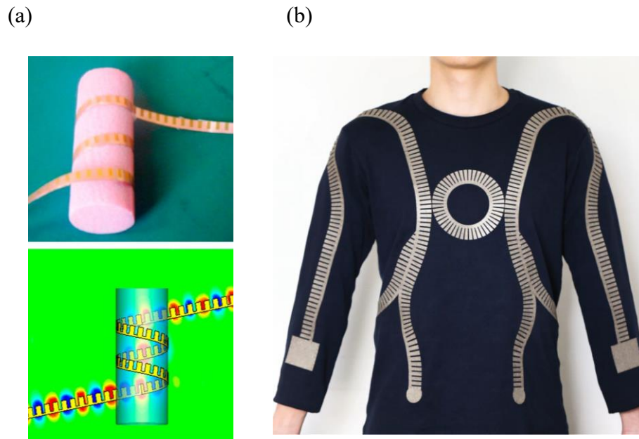
Figure 1.4 Applications of spoof SPPs. (a) Spoof SPP waveguides on flexible film. Reproduced from [25]. (b) Spoof plasmon textiles for wireless body sensor. Reproduced from [32].
