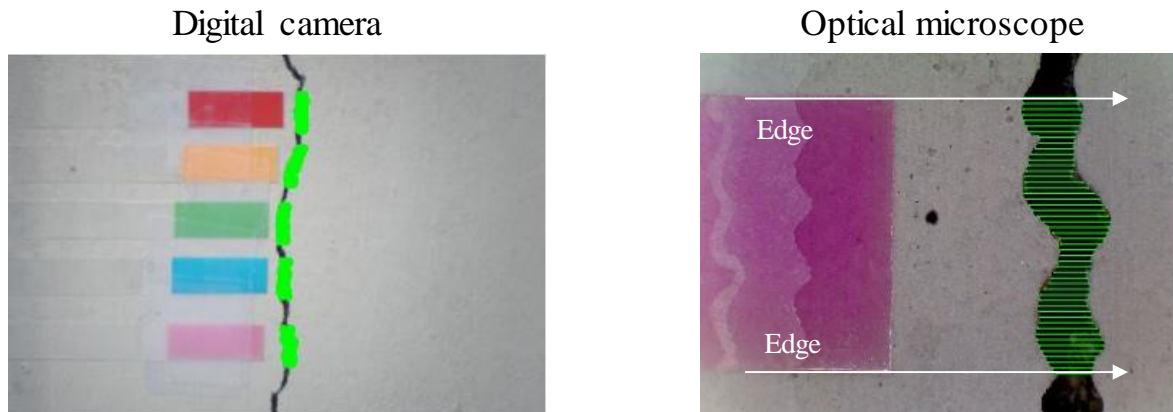
Fig. 5.9 Comparison of average crack width.
