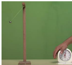
Figure 182. Count ten oscillations and stop the clock
